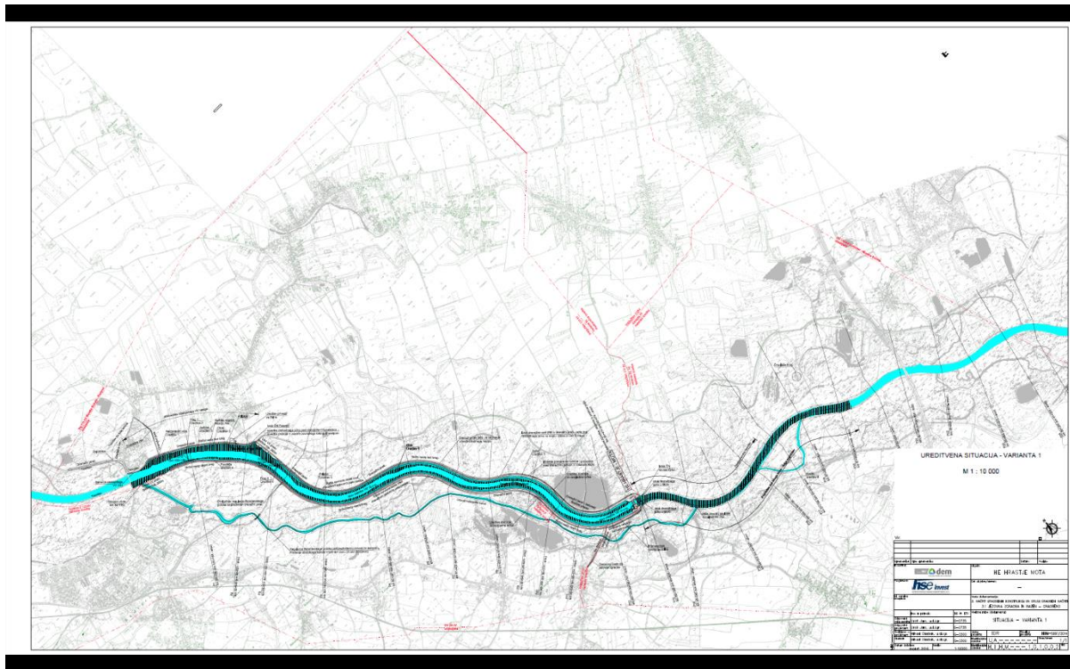
Figure 2. Variant 1 of the proposed hydroelectric power plant Hrastje-Mota on the uppermost Slovenian Mura. This variant depicts a 6.17 km long fish bypass channel with a yet-to-be defined discharge.
